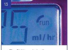
The RUN symbol will rotate to indicate that the pump is working
