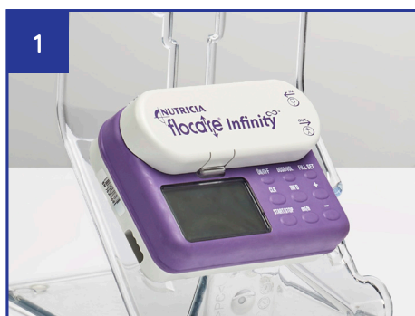
Attach Flocare Infinity pump to Z-Stand
