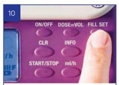
Press and hold FILL SET until beeps; to stop fill cycle press FILL SET again. **DO NOT OVERFILL**
