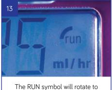
The RUN symbol will rotate to indicate that the pump is working
